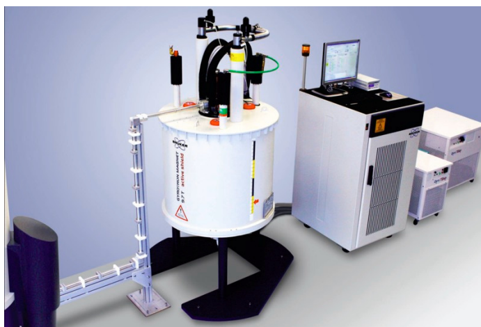
Fig. 1. The world's first commercially available solid-state NMR based on DNP technique
