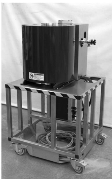
Figure 1: A mobile 400 MHz ( ^1\text{H} ) HTS magnet for high resolution spectroscopy
