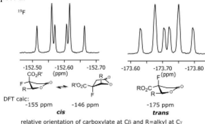
Fig. 1.  $^{19}\text{F}$  NMR signals for the two diastereomers and relevant ring conformations.
