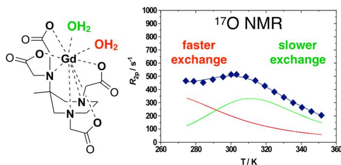
Fig.1. Different water exchange rates of the metal-bound water molecules in the Gd(AAZTA)(H<sub>2</sub>O)<sub>2</sub> complex.
