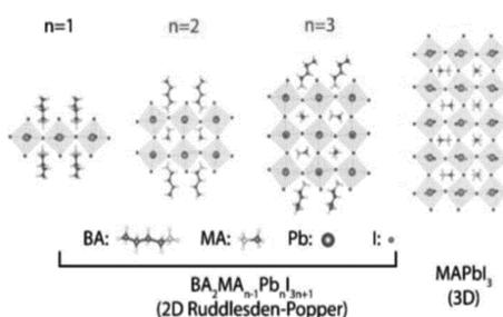
Fig. 1. Schematic structure of 2D RP perovskites  $BA_2MA_{n-1}Pb_nI_{3n+1}$  for  $n=1, 2, 3, 4$ , and of the corresponding 3D perovskites  $MAPbI_3$ . Here BA is butylammonium and MA is methylammonium.
