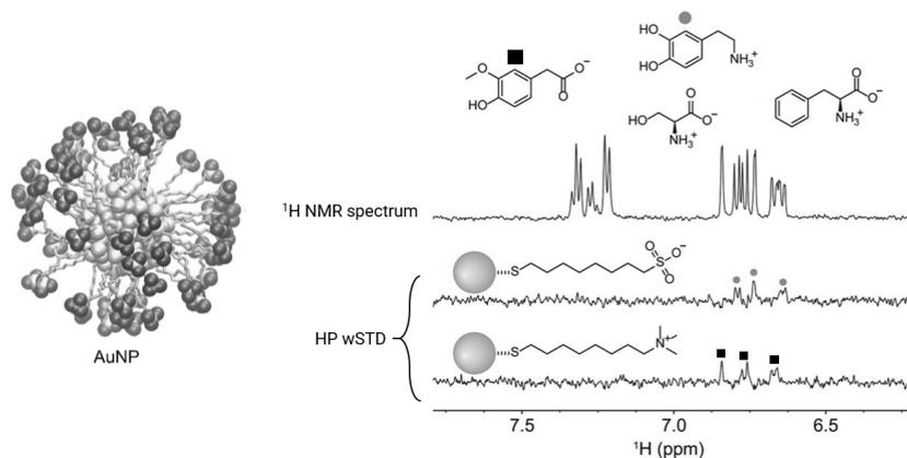
Fig. 1. Left: gold nanoparticle with sulfonated thiol ligand. Right: <sup>1</sup>H NMR spectrum of a mixture containing dopamine, homovanillic acid, L-phenylalanine and L-serine with the corresponding high-power water-assisted saturation transfer difference spectra (HP wSTD).
