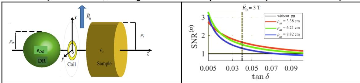
Fig. 1. Left panel: the DR sphere, circular RF Coil and cylindrical sample disposition considered in our full-wave electromagnetic model. Right panel: Normalised SNR calculated at 2 mm inside the first surface of the cylindrical sample along the  $z$  axis; values are normalized to the case without DR sphere. Different curves refer to DR spheres with  $\text{Re}(\epsilon_{\text{DR}}) = 1200$  and DR radii 3.38, 6.21, and 8.82 cm, supporting the  $L = 1, 3, 5$  resonant modes.
