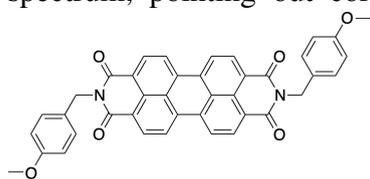
Moreover, variable temperature <sup>13</sup>C experiments provided information on the  $\pi$ -flip motion involving the methoxybenzyl substituents bonded to the imide nitrogen atoms,
