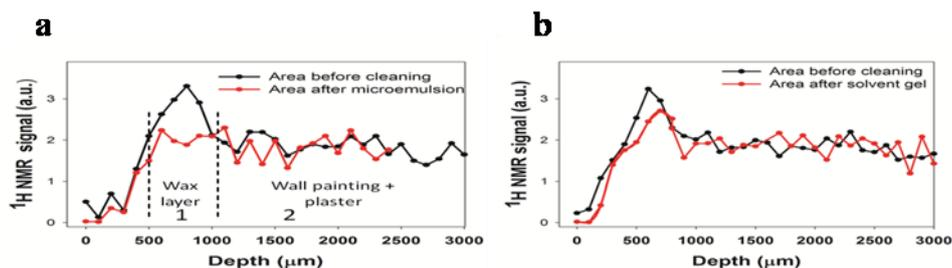
Fig. 1. Unilateral NMR was applied to evaluate the removal of the wax layer by two cleaning products: a micro-emulsion and a solvent gel. In figures 1a and 1b , the <sup>1</sup>H NMR depth profiles collected from two areas of painting were showed. In both areas before the cleaning treatments the NMR profile encoded two regions with a different hydrogen content.
