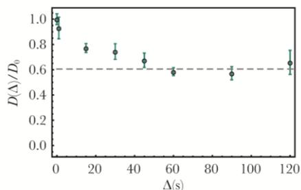
Fig. 1. The apparent diffusion coefficient of the singlet molecule in randomly packed spheres of diameter 500 – 600  $\mu\text{m}$ . The dashed line indicates the long-time, asymptotic value of the diffusion coefficient.
