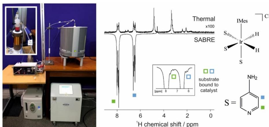
Fig. 1. Integrated flow system for SABRE hyperpolarization on a 1 T (43 MHz) benchtop NMR spectrometer (left) with example single-scan <sup>1</sup>H NMR spectra of 50 mM 4-aminopyridine acquired with and without SABRE hyperpolarization (right).
