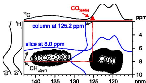
Fig. 2. CO<sub>2</sub> region of the <sup>1</sup>H-<sup>13</sup>C off-resonance FSLG HETCOR spectrum of POP loaded with 800 mbar of CO<sub>2</sub> highlighting the correlation between pyridinic CH<sub>α</sub> and adsorbed CO<sub>2</sub>.
