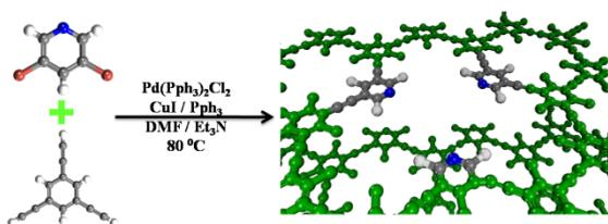
Fig. 1. Synthesis for the Pyridine POP with a structural model of a potential oligomer chain. Carbon (grey), oxygen (red), nitrogen (blue), hydrogen (white), repetitive part of the structure is shown in green.
