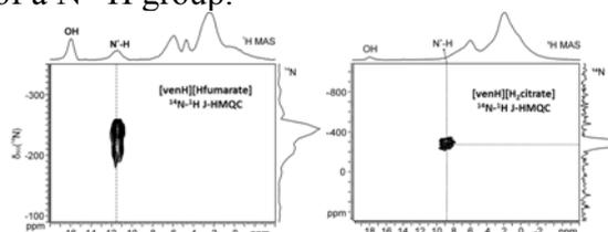
Fig. 1. 2D <sup>14</sup>N-<sup>1</sup>H J-HMQC spectra of [venH][HFumarate] and [venH][H<sub>2</sub>citrate] (<sup>1</sup>H Larmor frequency 600 MHz; MAS frequency 70 kHz)
