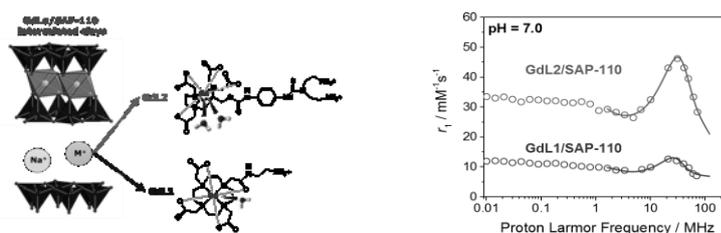
Fig. 1. (sx) Structure of GdLn/SAP-110 paramagnetic clays with the intercalated Gd<sup>3+</sup>-based complexes GdL1 and GdL2. (dx)  $1/T_1$  <sup>1</sup>H-NMRD profiles of GdLn/SAP-110.
