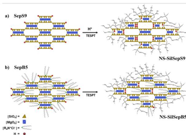
Fig. 1. Scheme for one-pot hybrid filler preparation from pure (sepS9) and organically modified sepiolite (SepB5) [1].
