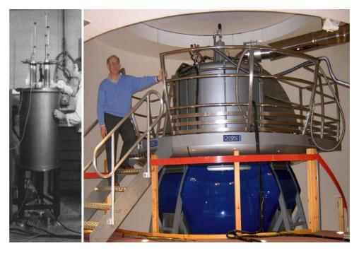
Fig. 2. Left: Picture of the early 270 MHz NMR spectrometer that Iain Campbell used at Oxford (photograph taken in 1971). Right: Iain standing next to a 950 MHz NMR spectrometer at Oxford (photograph taken in  $\sim$ 2008). (Colors are visible in the online version of the article; http://dx.doi.org/10.3233/BSI-130056.)
