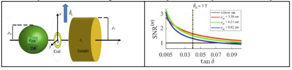
Fig. 1. Left panel: the DR sphere, circular RF Coil and cylindrical sample disposition considered in our full-wave electromagnetic model. Right panel: Normalised SNR calculated at 2 mm inside the first surface of the cylindrical sample along the *z* axis; values are normalized to the case without DR sphere. Different curves refer to DR spheres with  $Re(\epsilon_{DR})=1200$  and DR radii 3.38, 6.21, and 8.82 cm, supporting the L = 1, 3, 5 resonant modes.
