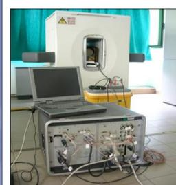
**NMR Porous Media Relaxometry:** sample were measured using a permanent magnet (0.8 T) and the analogical Console by Stellar (see picture on the left). The  $T_1$  distributions have been obtained by acquiring IR curves and using UpenWin [8] for the inversion of the data. In the right picture: the samples, which were cored as 20 mm diameter and measured using an home made 25.4 mm diameter coil: Lecce stone (up) and Uncastillo sandstone (down).
