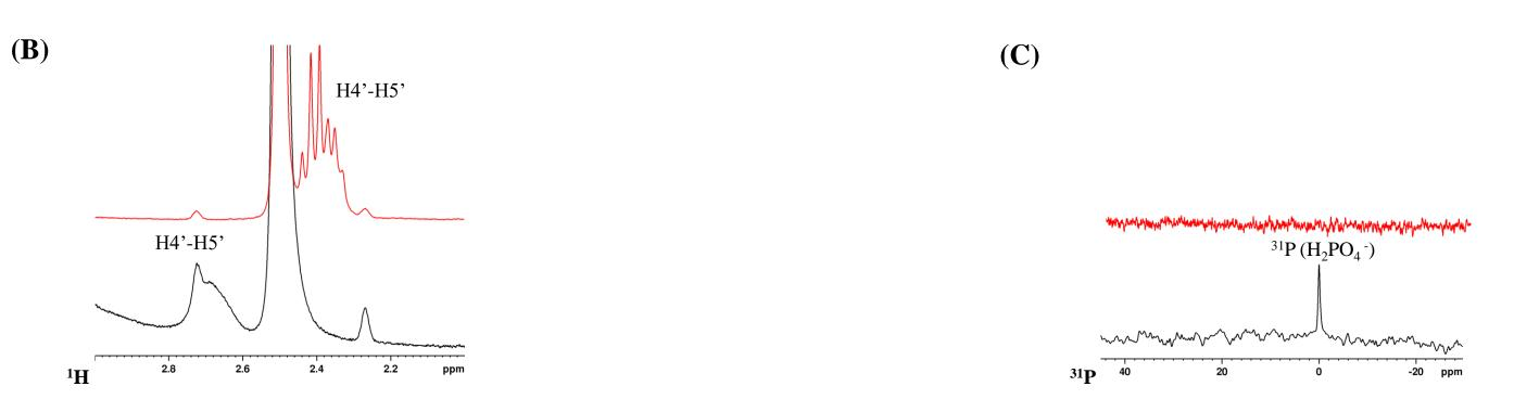
Overlay of 1D <sup>1</sup>H (**B**) and <sup>31</sup>P (**C**) NMR spectra of CQ (red) and CQDP (black).
