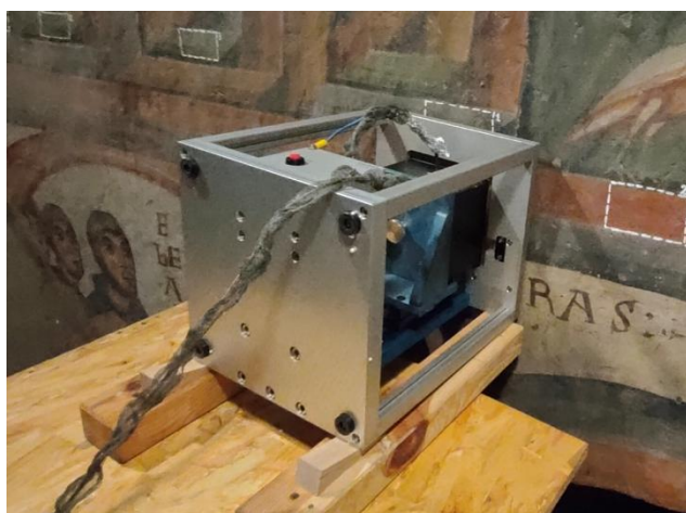
Fig. 1. Left: Experimental setup, the NMR-MOUSE is placed on a purposefully built structure to position its sensitive volume inside the wall paintings' surface. Right: Cumulative profiles (signal converted to water mass) acquired before and after treatment of a representative wall painting spot.
